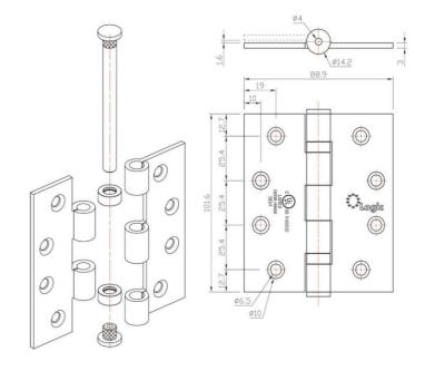
Material: SS304 Stainless Steel. Size - 4x3. x3.0mm-2BB. Recommendation - 3 Pcs Per Door. Door Weight Capacity - Up To 80kg. Application for wooden doors & metal doors Fixed Screws Bag: Wooden.
