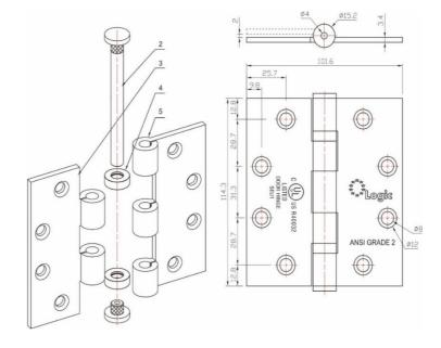
Material: SS304 Stainless Steel. Size - 4.5x4x3.4mm-2BB. Recommendation - 3 Pcs Per Door. Door weight capacity - up to 120kg. Application for wooden doors & metal doors
